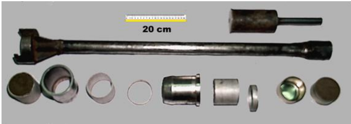
Figure 4.0. Soil sampling unit for determining soil bulk density.
