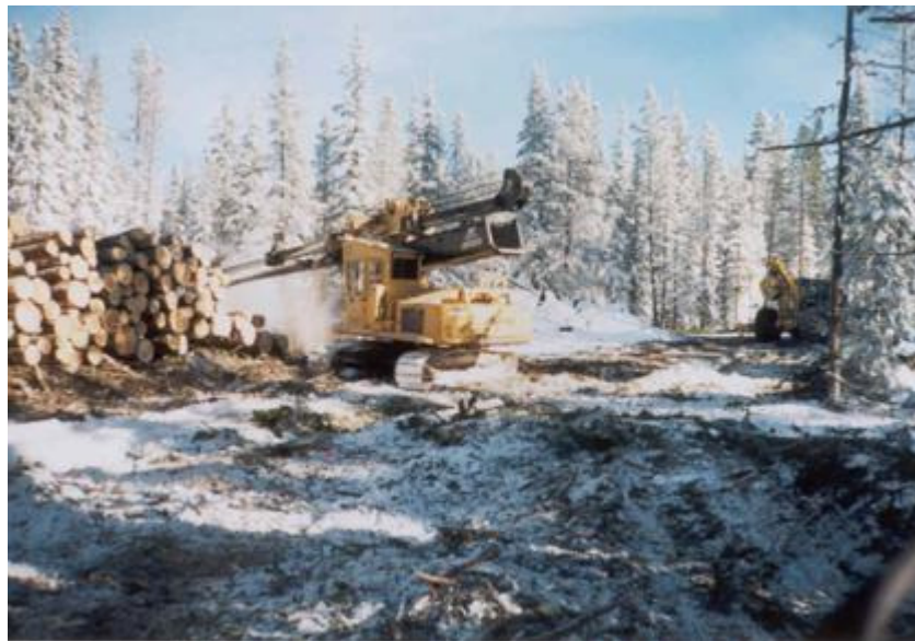
Photo 3. Conventional stroker / delimber and skidder working within Site #1 - Heller Creek.
